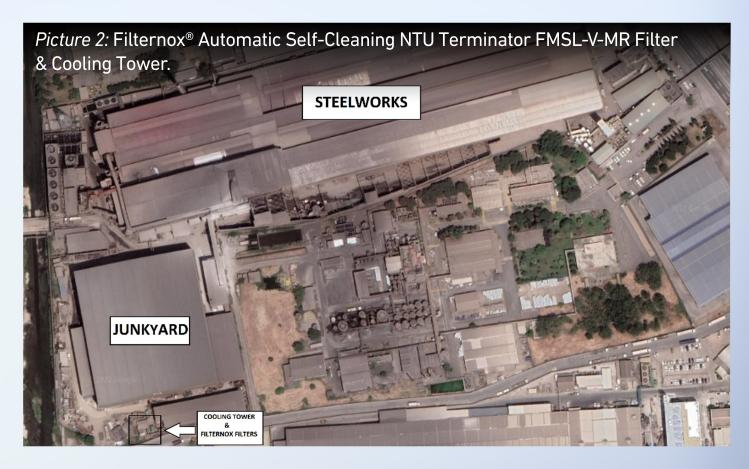
The location of the cooling tower is close to the steelworks of the factory and the junkyard. Therefore, the cooling water gets contaminated with iron and dust particles. (Picture 2)
