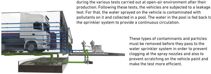
test. For that, the water sprayed on the vehicle is contaminated with pollutants on it and collected in a pool. The water in the pool is fed back to the sprinkler system to provide a continuous circulation. These types of contaminants and particles
