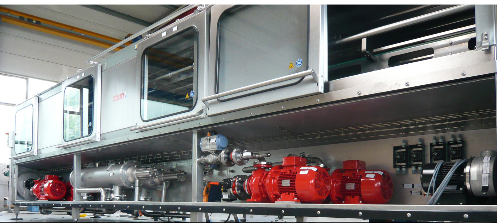
Industrial crate washer, protected by Filternox® automatic self-cleaning filters
