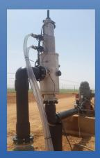
Application of Filternox<sup>®</sup> SPT-WBV-MR model filter for well water filtration.
