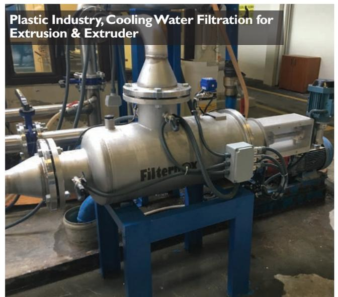
Plastic Industry, Cooling Water Filtration for Extrusion & Extruder
