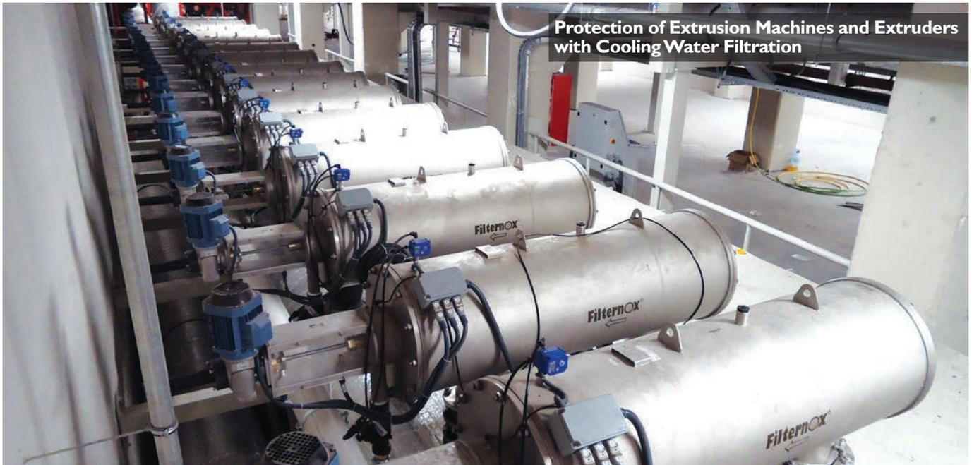
Protection of Extrusion Machines and Extruders with Cooling Water Filtration
