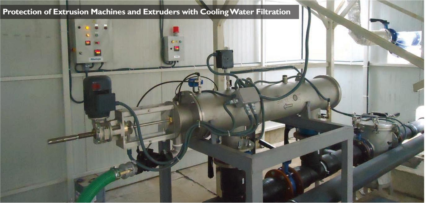
**Cooling Water Filtration For Welding Robots**
